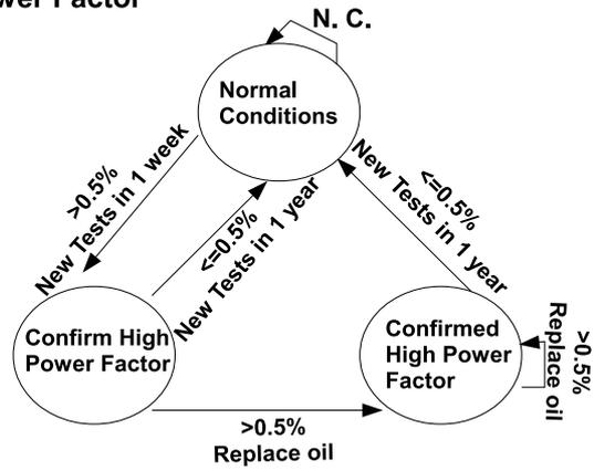
Fig. 3. FSM for the physical-chemical test.
