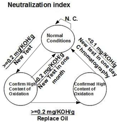
Fig. 2. FSM for the physical-chemical test.
