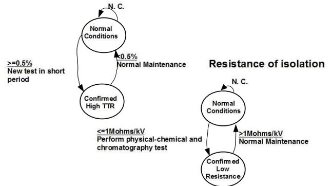
Fig. 4. FSM for the electrical test.
